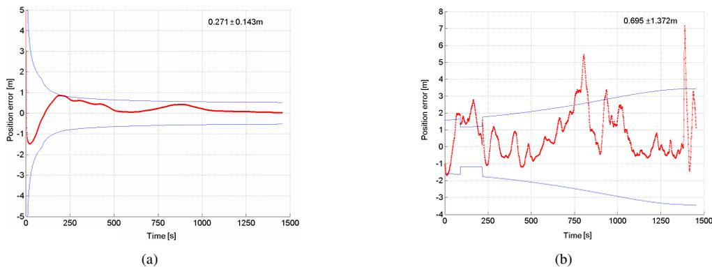
Figure 4. Double difference error using (a) Kalman filter and (b) least squares.
