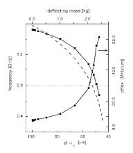
Resonant frequency and displacement sensitivity *df*, for insert #1 expressed in terms of the decreas dynamical gap x=  $d_0$ - $\delta_{max}$ . The dashed line refers calculated frequencies.
