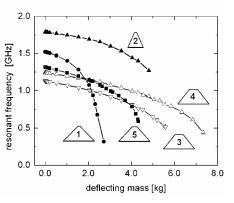
Dependence of measured frequencies for several inserts on the loading weight
