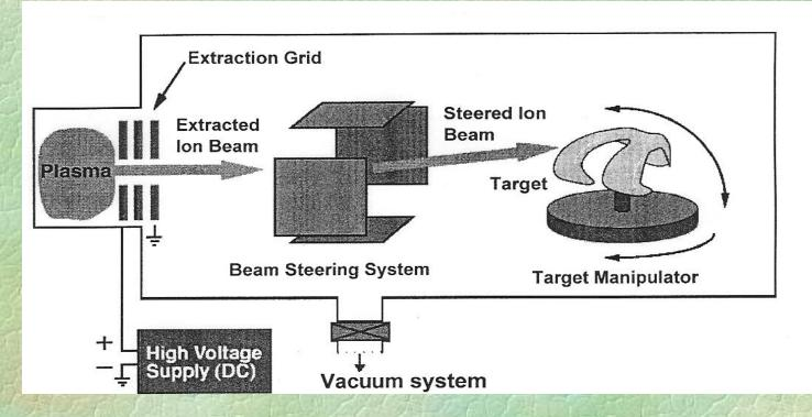
As a line-of-size, accelerator based, implantation technique beamline ion implantation has some shortcomings:
