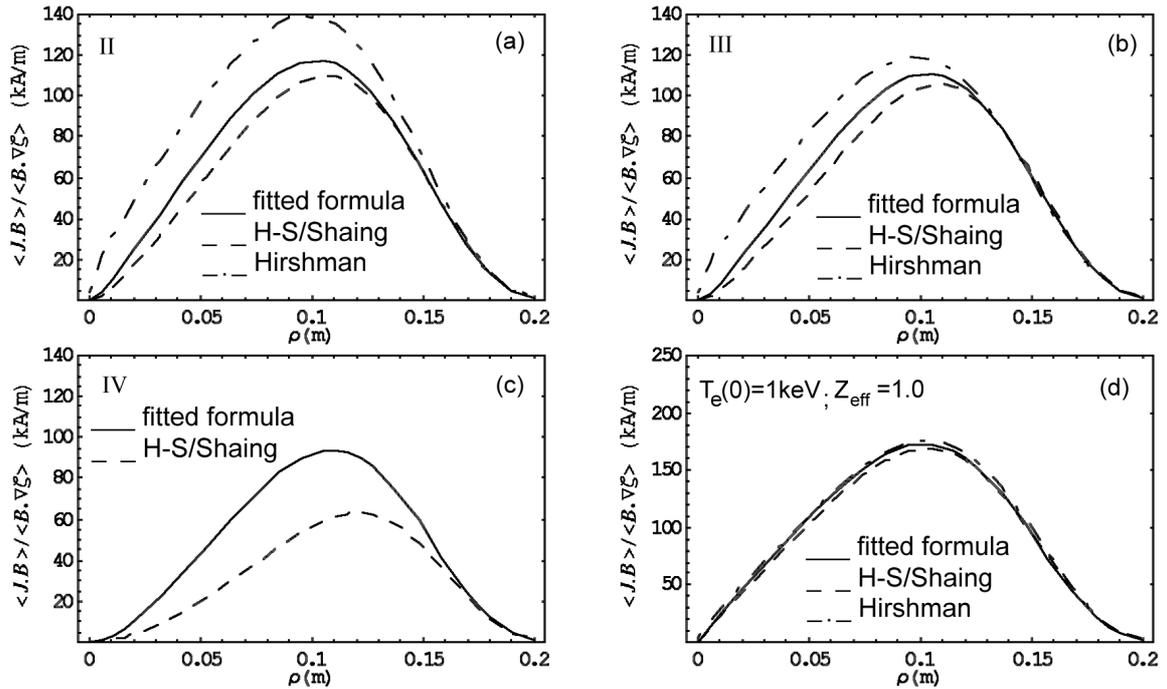
Figure 2: Bootstrap current profiles obtained from different models
