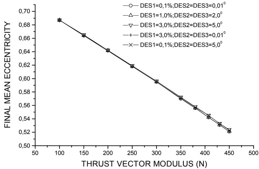
**Figure 6 – Final mean eccentricity vs. F, POW**
