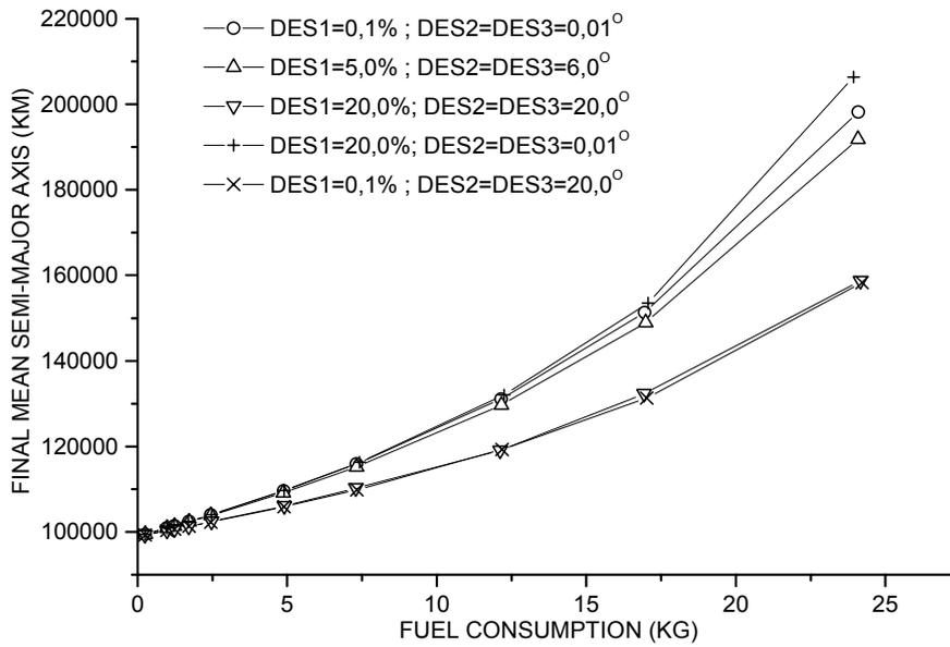
**Figure 1 – Final Mean Semi-major axis vs. Fuel Consumption , TOR**
