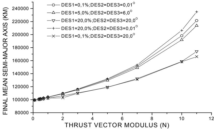
**Figure 3 – Final Mean Semi-major axis vs. F, TOR**
