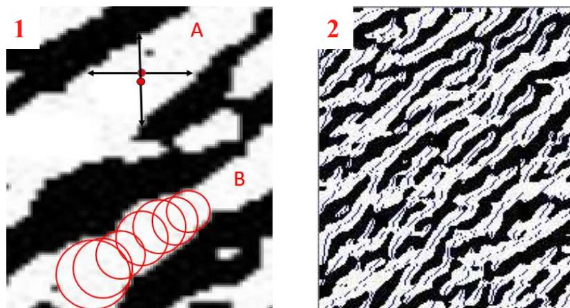
Figure 5: Methods tested to calculate the centerline of the wave crest 1: A Center of vertical and horizontal intervals, B center points of the circumferences circumscribed in the white objects (waves). 2: Image clipping with the centralized line obtained with method A.
