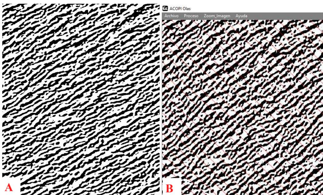
Figure 6: A, image clipping from the tested image, white objects representing the waves, black objects the background; B, image clipping from the software environment with profiles drawn in red.
