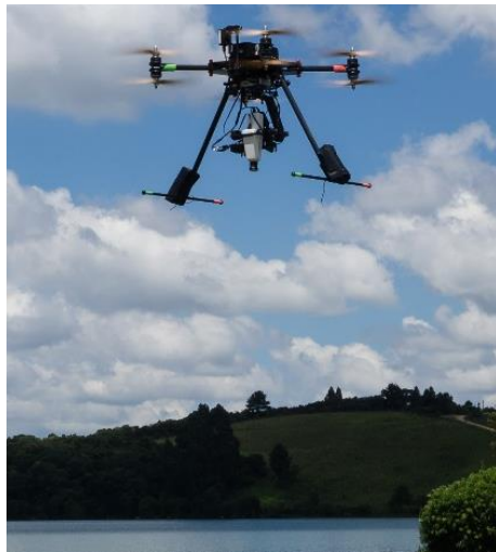
Figure 1: The sensor system is mounted on a coaxial octocopter. The cameras are stabilised by a two axis brushless gimbal.
