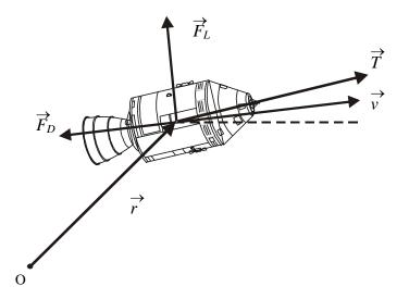
Fig. 1 - State variables, aerodynamic and thrust forces.
