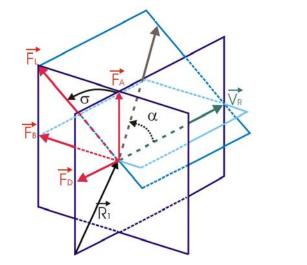
Fig. 2 - Components of the aerodynamic force, angle of attack  $\alpha$  the and bank angle  $\sigma$ .
