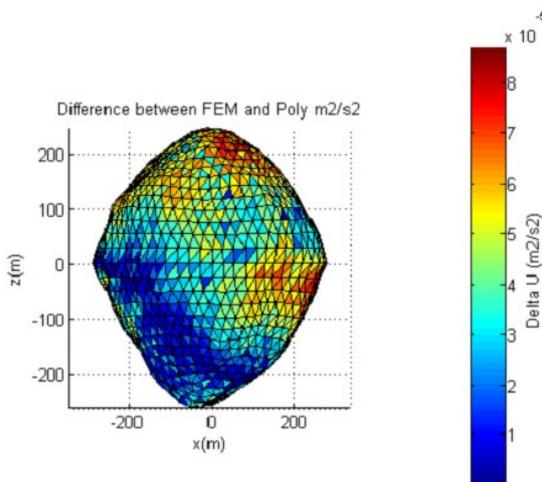
Figure 7. Potential difference over Benu surface (x-z view).
