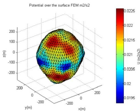
Figure 1. Potential over Bennu surface – FEM.
