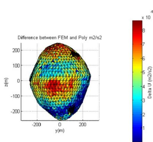
Figure 8. Potential difference over Benu surface (y-z view).
