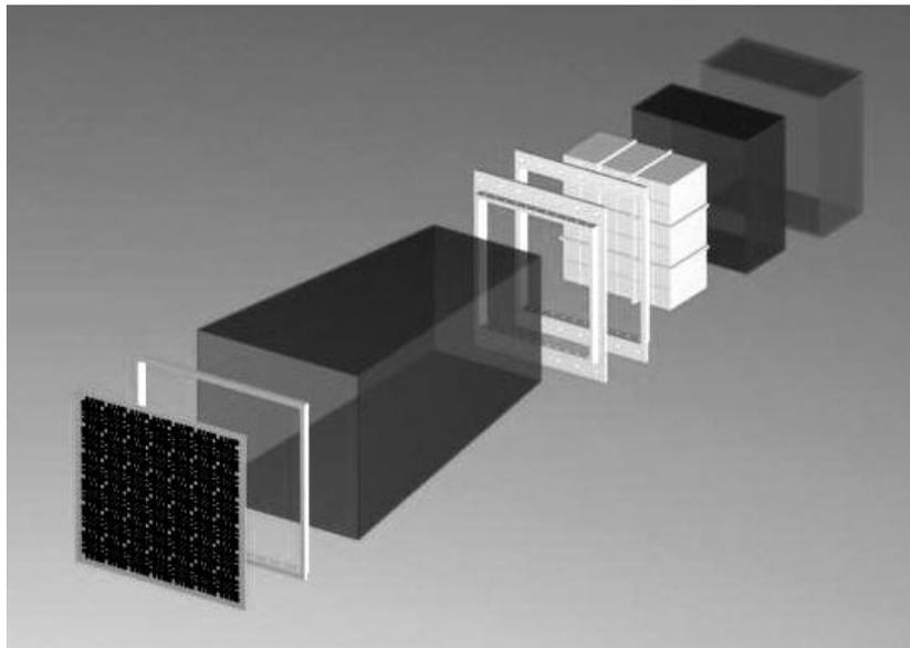
**Fig. 1.** Exploded diagram of the MIRAX hard X-ray camera. From left to right, the elements are: coded-mask, coded-mask support structure, Pb-Sn-Cu passive-shield walls, two structural flanges, detector modules, plastic scintillator and Pb-Sn-Cu passive shield.
