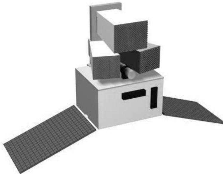
**Fig. 3.** A preliminary view of the MIRAX spacecraft. The two cameras mounted over the satellite bus are the hard X-ray cameras (CXDs), whereas the soft X-ray camera is on top of the CXDs. The APS optical star camera is placed in between the CXDs. The external dimensions are approximately 1.5 m x 0.7 m x 0.7 m (with the solar panels folded over the spacecraft).
