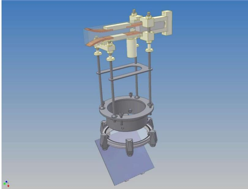
*Figure 2 - The model of the developed HFB-PPT (top) mounted on its support (center) with a mirror on the bottom for instrumentation purposes.*
