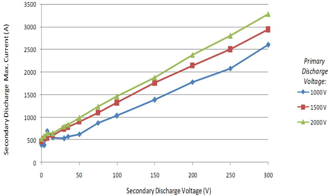
Figure 10. – Maximum Current in the secondary discharge as a function of the secondary discharge voltage for three different primary discharge voltages.
