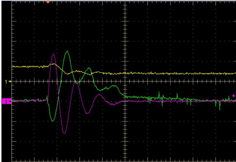
Figure 5. – Second regimen. Typical discharge for secondary discharge voltage of 50V (with primary discharge voltage of 1.5 kV) and between 30 and 75 V (with primary discharge voltage of 2 kV) – not observed at 1 kV-, showing the secondary discharge capacitor voltage (yellow, 100V/div), secondary discharge current (green, 500 A/div) and primary discharge current (pink, 5000 A/div) at 100  $\mu$ s/div (horizontally). Taken with 2kV primary discharge and 75 V secondary discharge.
