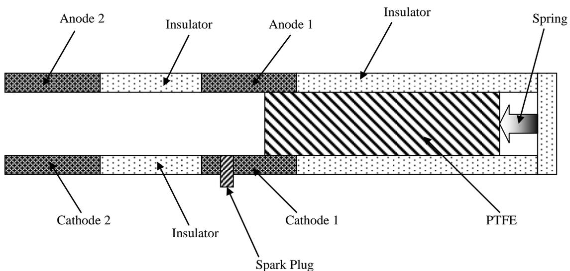
Figure 1 – HFB-PPT Discharge Chamber.
