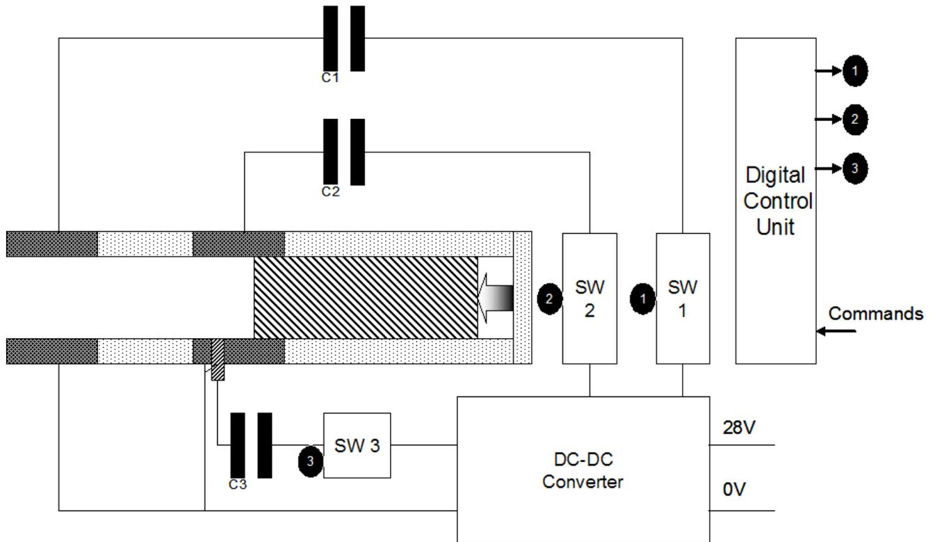
Figure 3 – A block diagram of the HFB-PPT.
