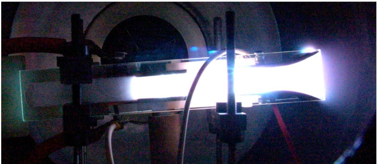
Figure 11. – HFB-PPT firing.
