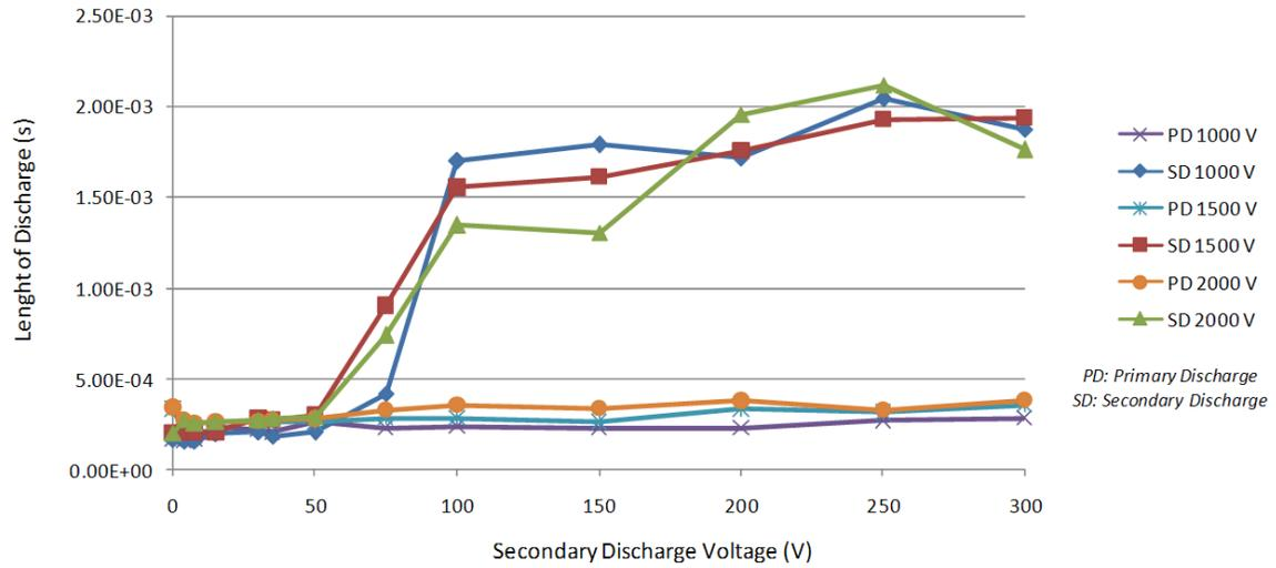
Figure 8. - Length of the secondary discharge as a function of the voltage applied in the secondary electrodes for three different primary discharge voltages.
