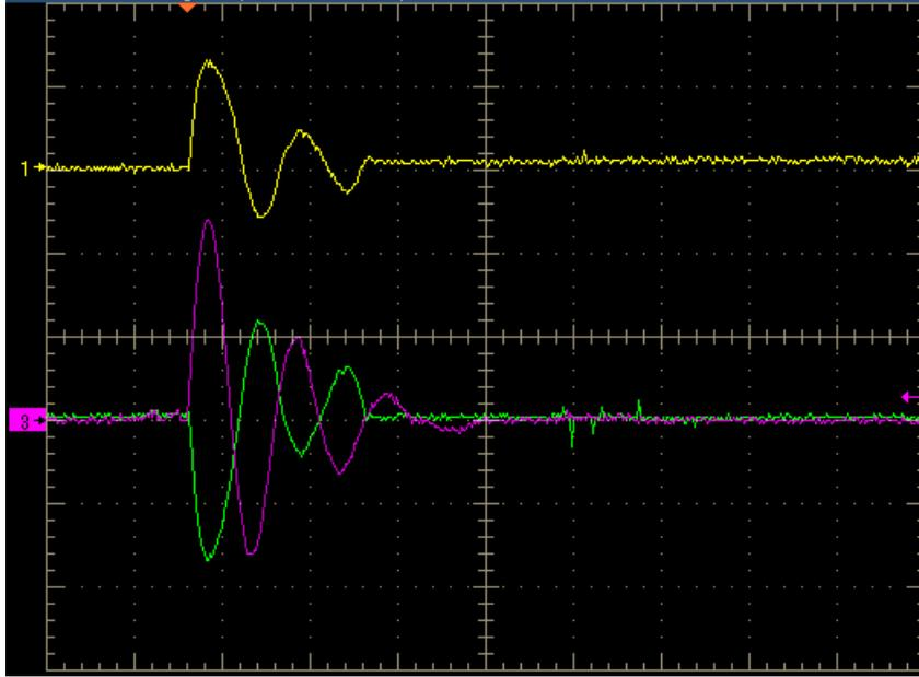
Figure 4. – First regimen. Typical discharge for secondary discharge voltages between 0 and 50V (with primary discharge voltage of 1 kV or 1.5 kV) and between 0 and 15 V (with primary discharge voltage of 2 kV), showing the secondary discharge capacitor voltage (yellow, 100V/div), secondary discharge current (green, 500 A/div) and primary discharge current (pink, 2000 A/div) at 100  $\mu$ s/div (horizontally). Taken with 2 kV primary discharge and 0 V secondary discharge.
