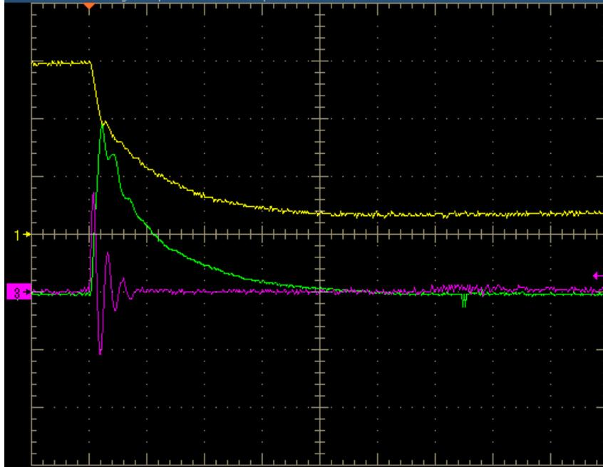
Figure 7. – Fourth regimen. Typical discharge for secondary discharge voltages above 150 V (for 1 kV main discharge), 200 V (for 1.5 kV main discharge) or 250 V (for 2 kV main discharge), showing the secondary discharge capacitor voltage (yellow, 100V/div), secondary discharge current (green, 1000 A/div) and primary discharge current (pink, 5000 A/div) at 100  $\mu$ s/div (horizontally). Taken with 1.5kV primary discharge and 300 V secondary discharge.
