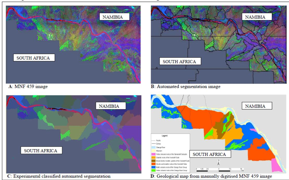
Figure 3: Un-scaled experimental results of image segmentation. The diagram (A) shows the MNF459 Hymap image used in the automated segmentation process, with the segmentation results shown by diagram (B). The diagram (C) shows the results from the classified image obtained from automated segmentation while diagram (D) shows the geological map derived by an expert from the manual digitising of a Hymap MNF 459 image.
