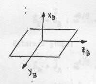
$$\vec{J}_{B} = I_{B}^{\star} \hat{x}_{B} \hat{x}_{B} + I_{B}^{\dagger} \hat{y}_{B} \hat{y}_{B} + I_{B}^{\dagger \dagger} \hat{z}_{B} \hat{z}_{B}$$
