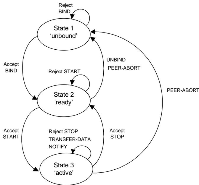
**Figure 2-4: Simplified RAF Service Provider State Transition Diagram**
