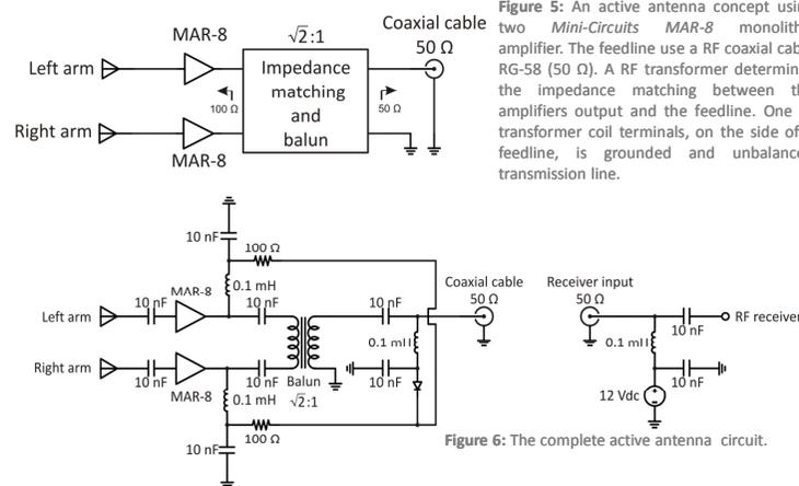
Figure 5: An active antenna concept using two Mini-Circuits MAR-8 monolithic amplifier. The feedline use a RF coaxial cable RG-58 (50 Ohm). A RF transformer determines the impedance matching between the amplifiers output and the feedline. One of transformer coil terminals, on the side of a feedline, is grounded and unbalanced transmission line.
