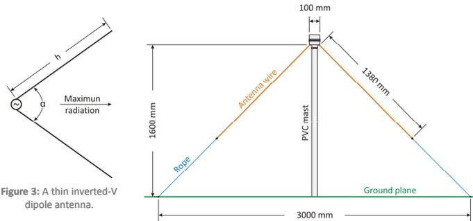
Figure 3: A thin inverted-V dipole antenna.
