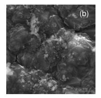
Fig.1. SEM images of BDD films (a) before and (b) after the deposition of copper nanoparticles.
