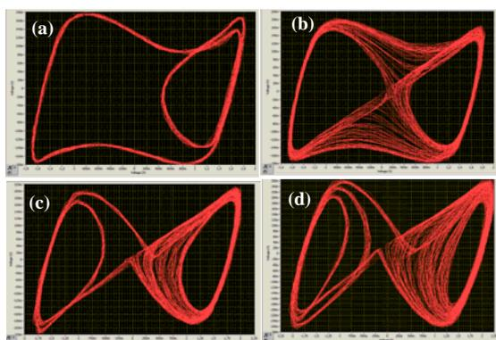
Figure 3 – Four experimental attractors for the implemented chaotic circuit. See the similarities between the attractors (a) and (b) with the theoretical attractors (a) and (b) in Fig. 2.
