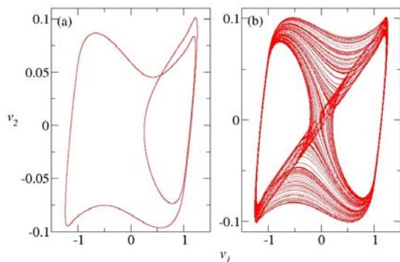
Figure 2 – Theoretical (a) periodic and (b) chaotic attractors for the parameter values of the two green marks 'a' and 'b' in Fig. 1. The axes are in voltage units (Volts).
