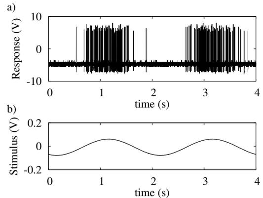
**Figure 1 – Circuit response (a) to a sinusoidal stimulus (b). Note the stochastic nature of the response.**
