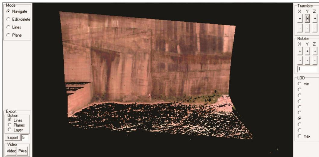
Figure 4. Outcrop Explorer's visualization and navigation module. Note the high quality of the details of the rockface as evidenced by the zig-zag lines (stratifications) in the upper left corner of the point cloud, enhanced by weathering (darker areas of the wall).
