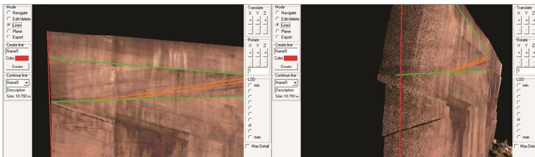
Figure 6. Interpretation lines revealing a cross-stratification directly on the digital model. Colors can be changed to enhance hierarchy or specific features. Note that lines are attached with the points as shown by the rotation of the digital model.
