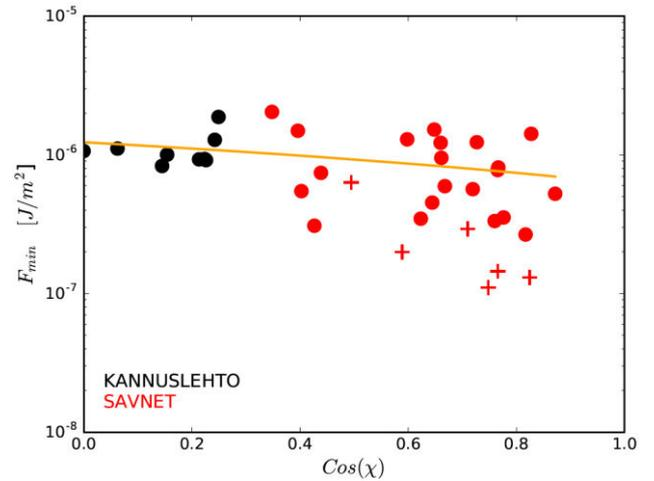
**Figure 4.** Values of  $F_{\min}$  obtained by using the Kannuslehto (black) and the SAVNET (red) receiver systems, evaluated against the cosine of the average solar zenith angle of the VLF propagation paths. The crosses refer to events occurred during solar minimum and filled circles to events occurred during solar maximum. The yellow line is the linear fit considering the events occurred during solar maximum.
