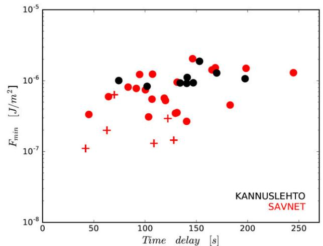
**Figure 5.** Values of  $F_{\min}$  obtained using the Kannuslehto (black) and the SAVNET (red) receiver systems, evaluated against the time delay between the onset of the X-ray flare and the beginning of the VLF amplitude
