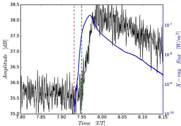
**Figure 1.** Temporal behaviour of the amplitude of a VLF signal recorded at Kannuslehto (black line) and the temporal variation of the X-ray flux with wavelength less than  $2 \text{ \AA}$  (blue line). The vertical dashed red and green lines represent the initial time of the flare and the start time of the VLF amplitude deviation, respectively.
