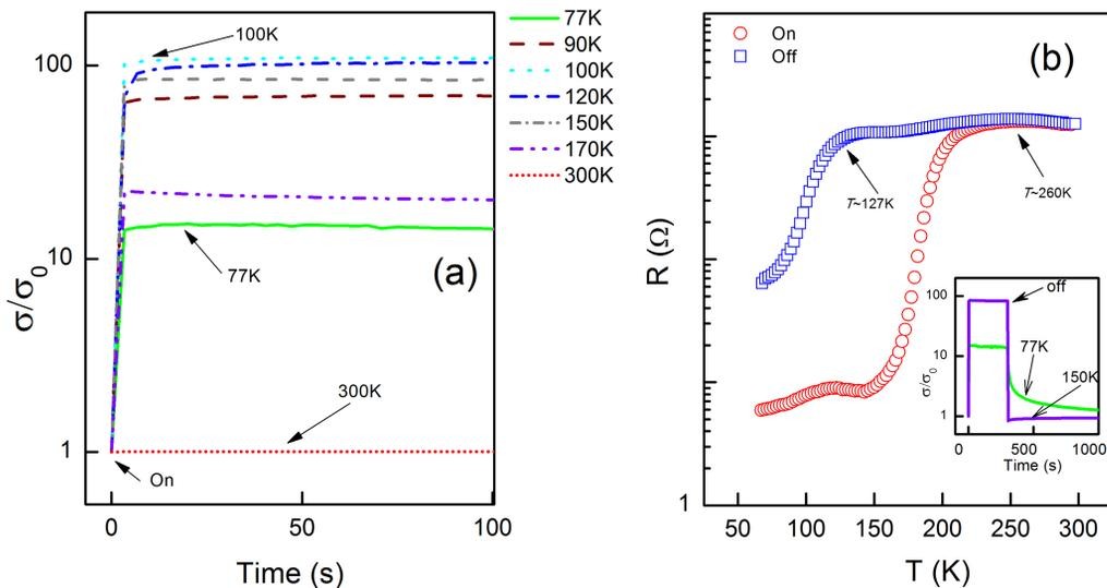
**Figure 2.** (a) Presents the normalized photoconduction under IR irradiation, for temperatures in the range 300-77K. (b) The resistance in function of temperature showing the change of conduction channel from the barrier to the well, the insert I contain the behavior of conductivity when the LED is on and off, for temperatures of 77K and 150K.
