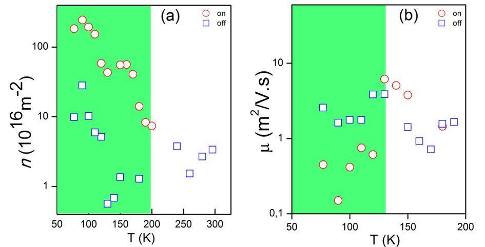
**Figure 4.** Presents the data found with Hall measurements in the 6072 sample, (a) the charge density and (b) the carrier mobility, with and without illumination.
