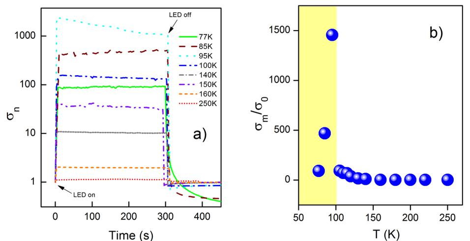
**Figure 5.** (a) Presents the normalized photoconductivity, when LED is turn on and off for. (b) The peak of normalized photoconductivity under IR irradiation in function of temperature. Those data is for 7111 sample and temperatures are in the range of 300-77K.
