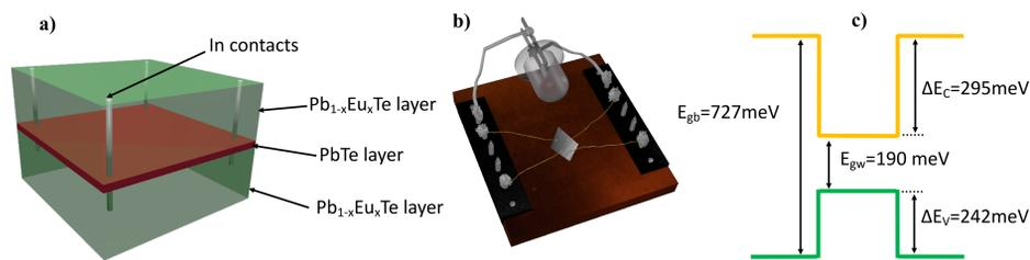
**Figure 1.** Illustration of (a) PbTe/Pb<sub>1-x</sub>Eu<sub>x</sub>Te QW with In contacts. (b) sample port with a sample connected with gold thin wires and a LED. (c) energy band diagram in units of meV, where  $E_{gb}$  is the energy gap of barrier,  $E_{gw}$  is the energy gap of the well,  $\Delta E_v$  and  $\Delta E_c$  are the energy high of valence and conduction band respectively.
