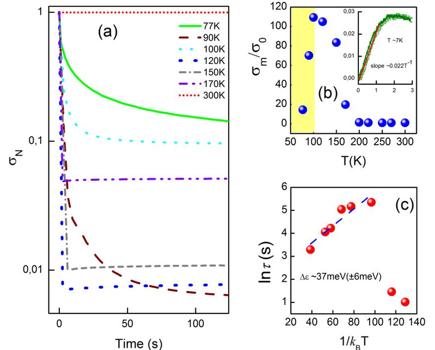
**Figure 3.** (a) Normalized photodecay, when LED is turn off for 6072 sample and (b) the peak of normalized photoconductivity under IR irradiation in function of temperature in the range of 300-77K, the inset shows the slope of the magnetoresistance curve for Pb<sub>0.88</sub>Eu<sub>0.12</sub>Te film with 2.3μm of thickness and (c) decay time in function of  $1/k_B T$  and linear fit, getting the activation energy for this film.
