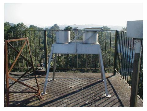
Figure 1b – Photo of wet-only collector (brand MTX - Italy) installed atop of the water tank at PEFI (Forti, 2000).
