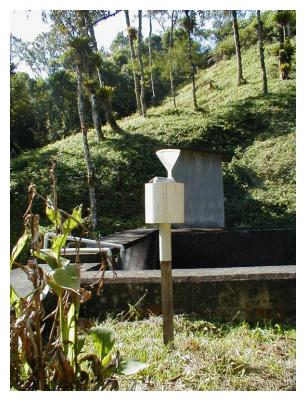
Figure 1a – Picture of the bulk collector installed next to the catchment B weir at CUNHA (Forti, 2000).
