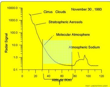
The figure shows an example of INPE's Lidar signal. The signal is blocked from 0 to 12 km. Cirrus clouds and stratospheric aerosols overlap the atmospheric molecular signal from 15 to 30 km. Resonant scattering of sodium are obtained from 78 to 105 km. From 30 to 75 km clean molecular Rayleigh signal is used to measure the atmospheric density and temperature.
