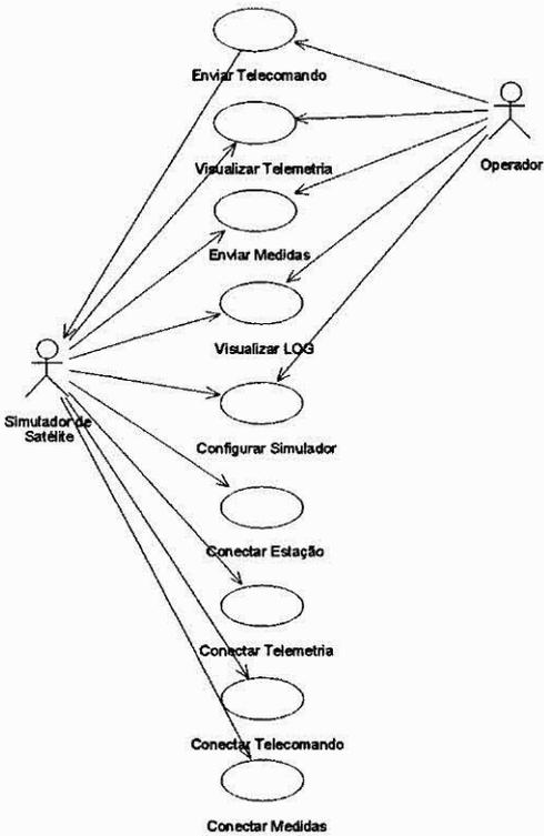
**Figure2 – Use Case Diagram : Simulator Subsystem**
