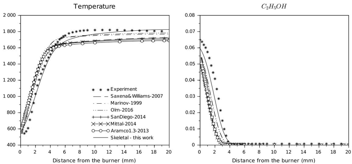
**Fig. 4** Temperature and fuel mole fraction for different mechanisms against experimental data from [13] at  $\phi = 1.0$ . Results are for a burner-stabilized flat flame with initial temperature  $T_u = 560 K$  and atmospheric pressure
