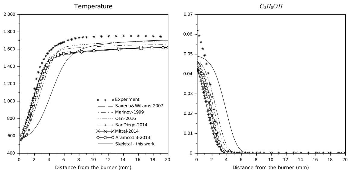
**Fig. 6** Temperature and fuel mole fraction for different mechanisms against experimental data from [13] at  $\phi = 0.75$ . Results are for a burner-stabilized flat flame with initial temperature  $T_u = 560$  K and atmospheric pressure
