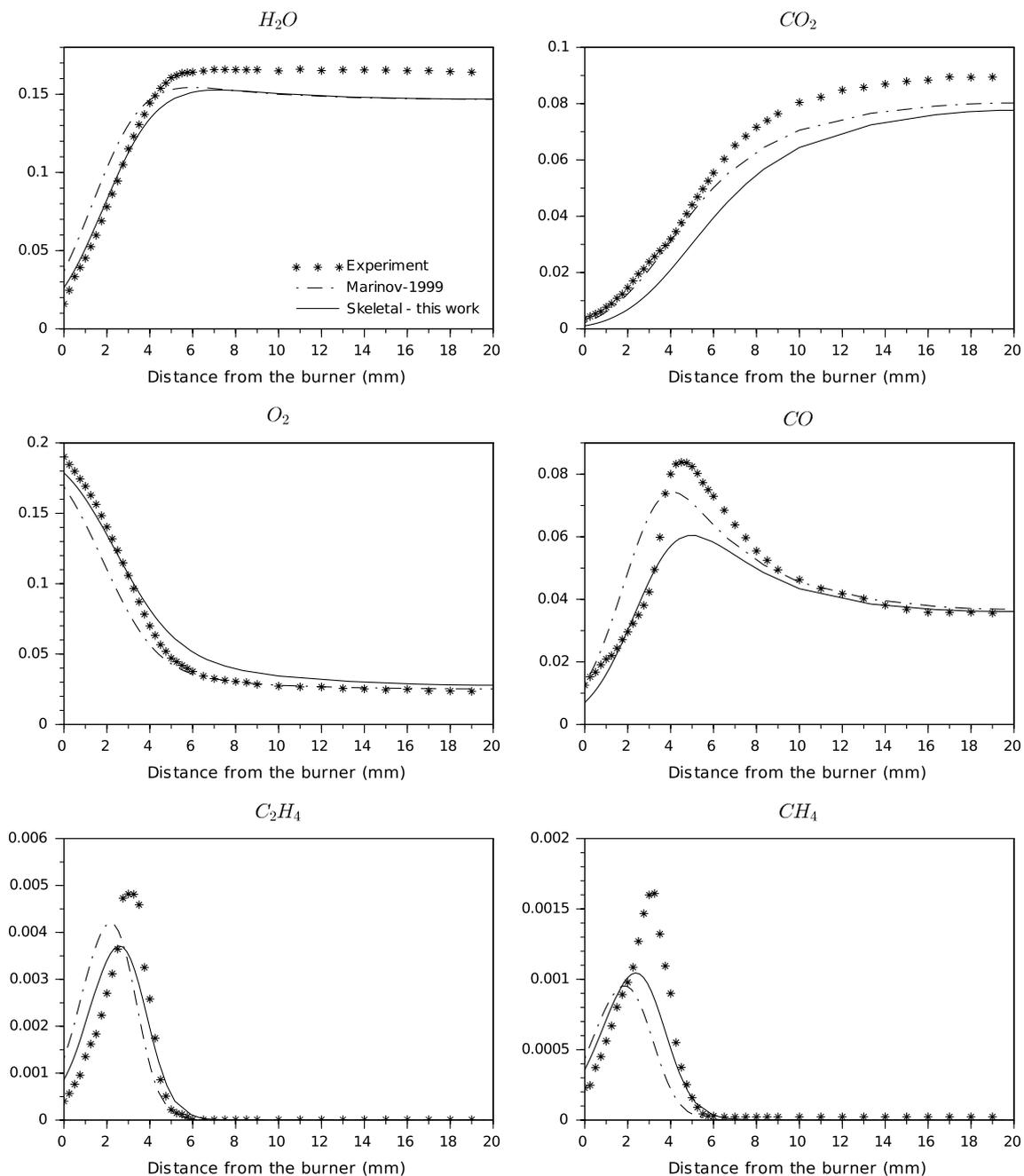
**Fig. 7** Species mole fractions for detailed and skeletal mechanisms against experiment data from [13] at  $\phi = 1.0$ . Results are for a burner-stabilized flat flame with initial temperature  $T_u = 560$  K and atmospheric pressure
