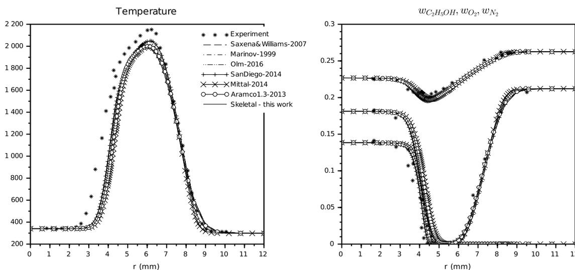
**Fig. 11** Temperature and species mass fractions of fuel, oxidizer and nitrogen for different mechanisms for a premixed counterflow flame, compared with measurements [32]. The boundary conditions are given in Table 3
