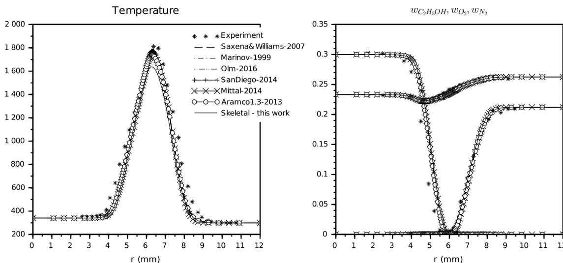
**Fig. 10** Temperature and species mass fractions of fuel, oxidizer and nitrogen for different mechanisms for a non-premixed counterflow flame, compared with measurements [32]. The boundary conditions are given in Table 3
