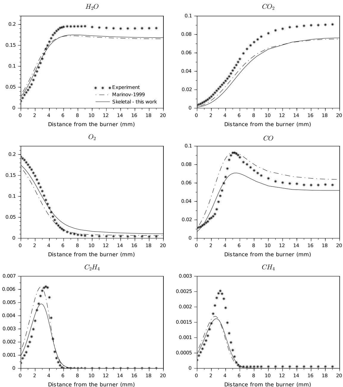
**Fig. 8** Species mole fractions for detailed and skeletal mechanisms against experiment data from [13] at  $\phi = 1.25$ . Results are for a burner-stabilized flat flame with initial temperature  $T_u = 560$  K and atmospheric pressure
