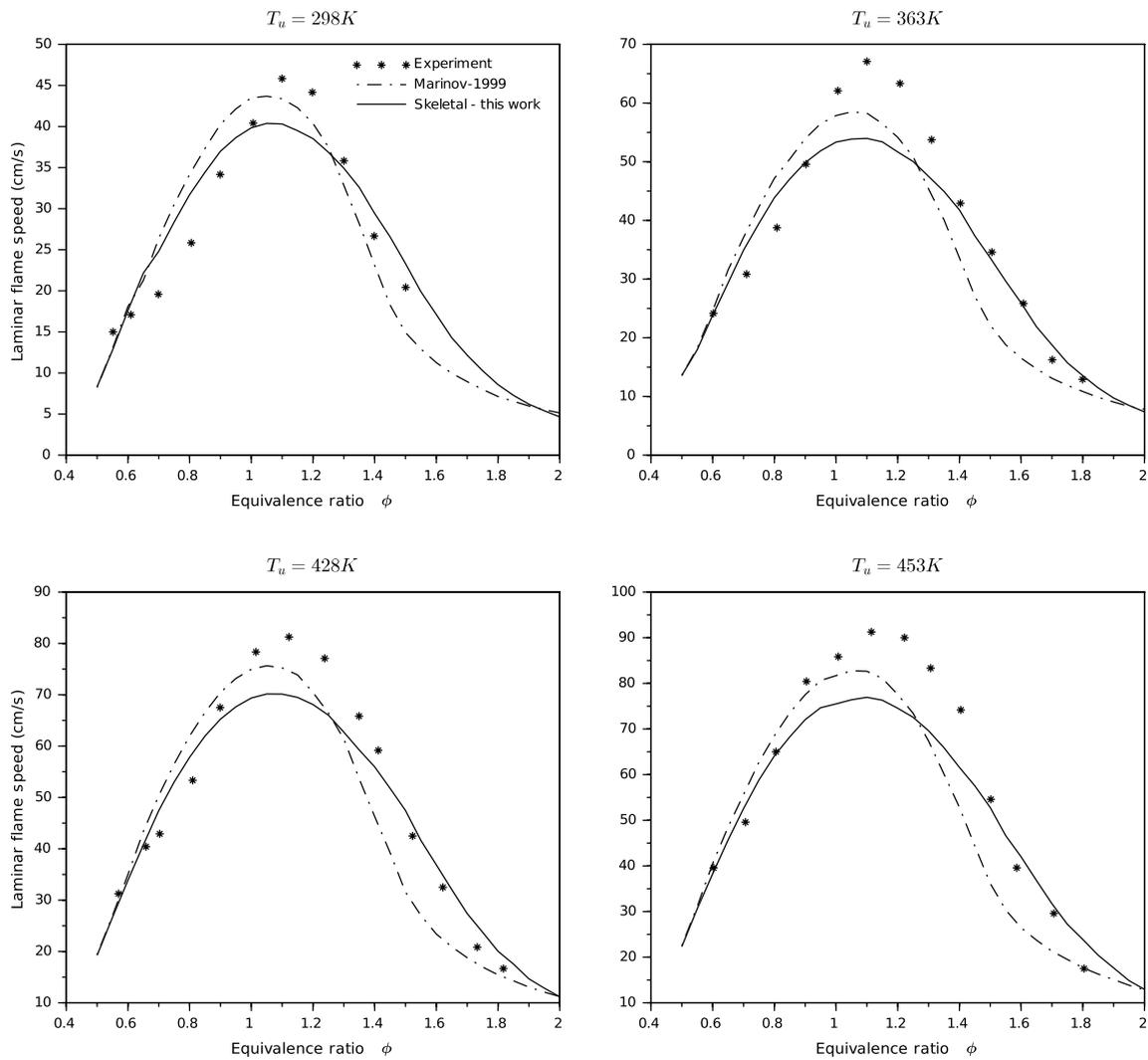
**Fig. 3** Laminar flame speed calculated in a freely propagating flat flame for ethanol for different initial temperatures. The result of the skeletal mechanism is compared with different mechanisms in the literature and experimental data [8]
