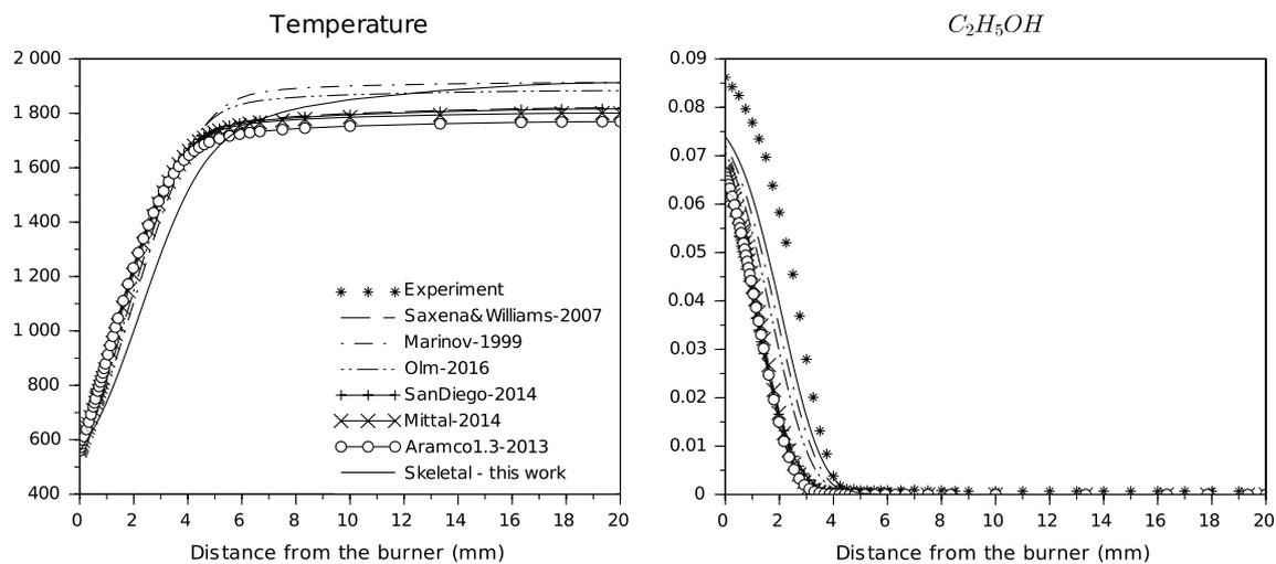
**Fig. 5** Temperature and fuel mole fraction for different mechanisms against experimental data from [13] at  $\phi = 1.25$ . Results are for a burner-stabilized flat flame with initial temperature  $T_u = 560$  K and atmospheric pressure
