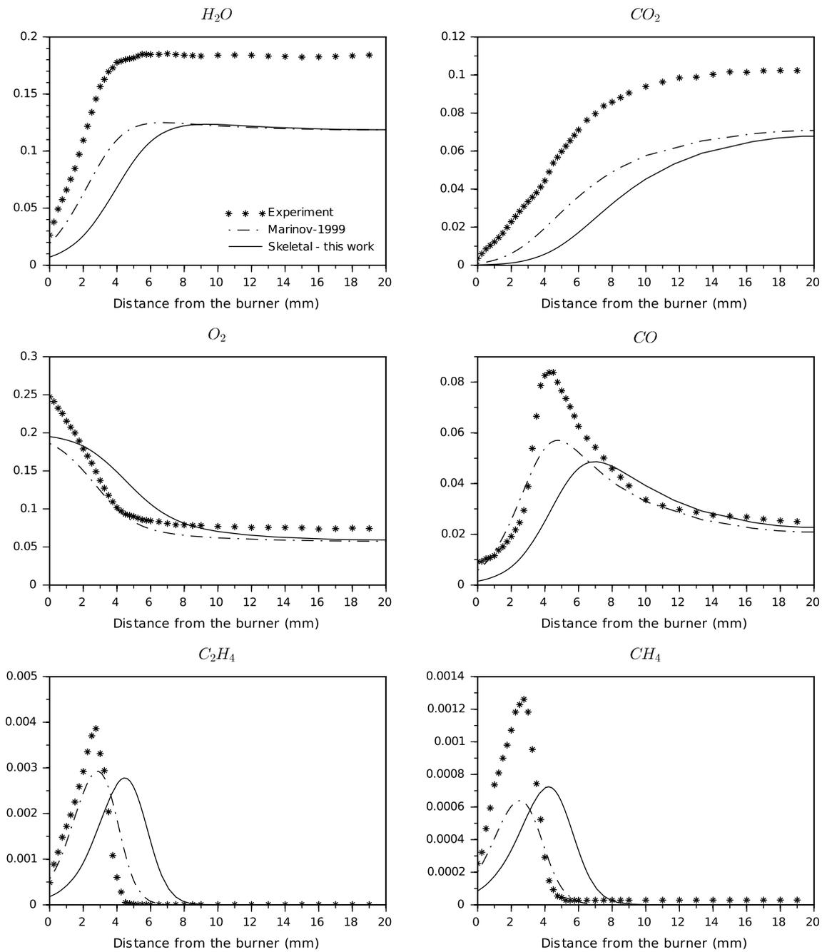
**Fig. 9** Species mole fractions for detailed and skeletal mechanisms against experiment data from [13] at  $\phi = 0.75$ . Results are for a burner-stabilized flat flame with initial temperature  $T_u = 560$  K and atmospheric pressure
