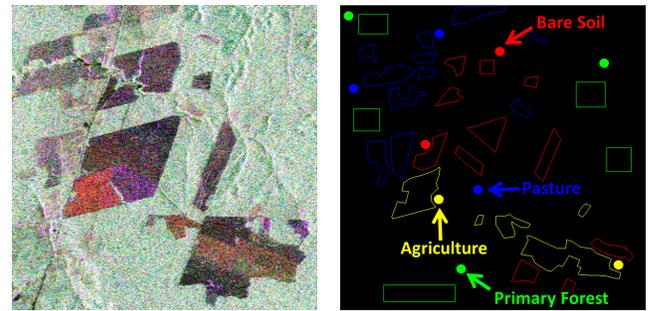
(a) ALOS/PALSAR image (b) Training samples (solid circles) in R(HH)G(HV)B(VV) color and validation samples (empty polygons)
