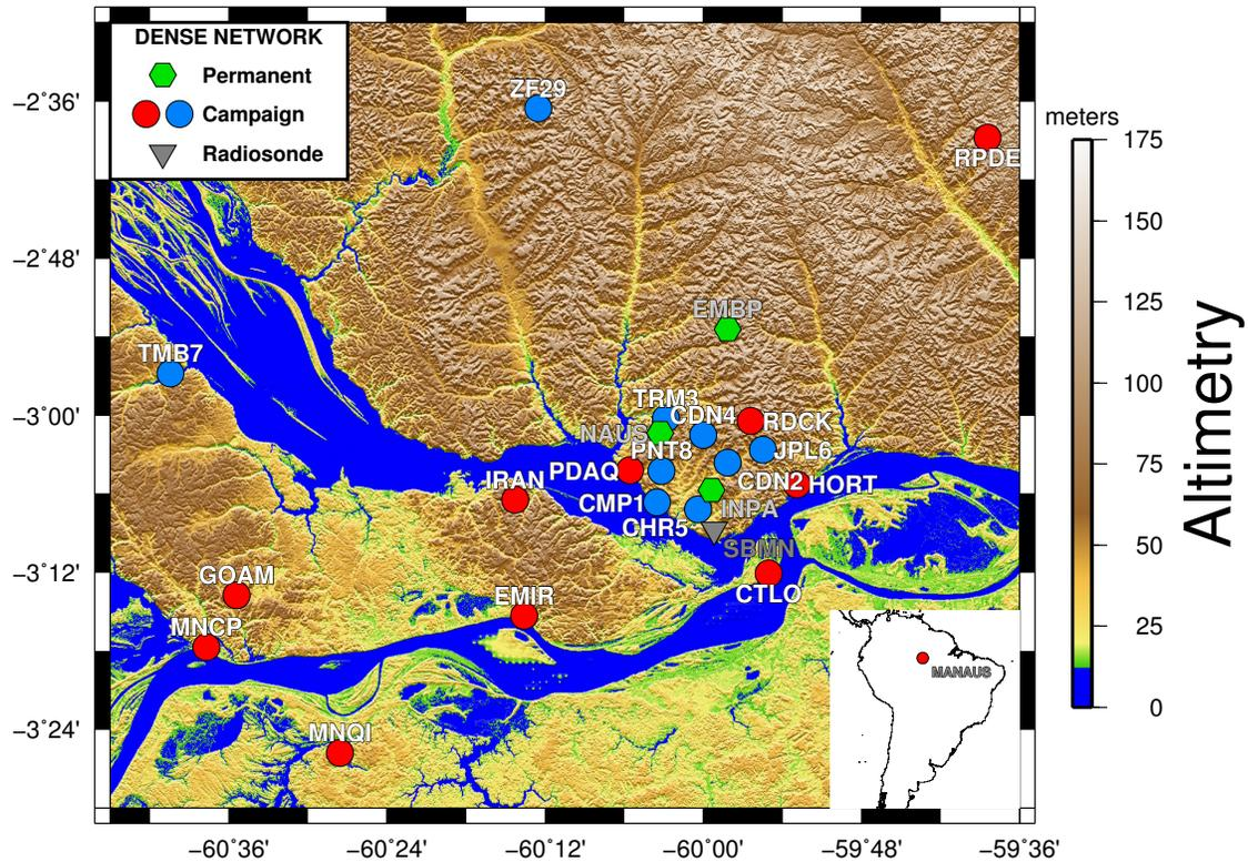
FIG. 2. Map of the Manaus Dense GNSS Meteorological Network, April 2011 - April 2012. Green and blue stations were present for the duration of the experiment. Red stations were present from August 2011 to April 2012. SBMN (82332) is the site for twice daily radiosondes and represents the tip of the Manaus “peninsula”.
