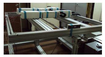
Fig. 17. Both heat pipes installed on the table.
